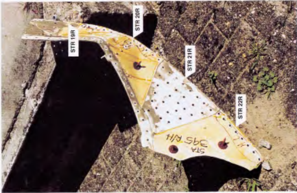
Fig. 14 Section of the STA 395 bulkhead (RH-side)
